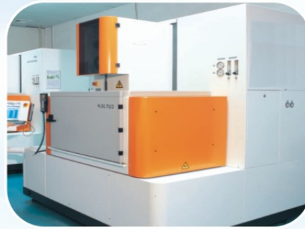
慢走絲車間 Slow-feed Wire Cutting workshop
